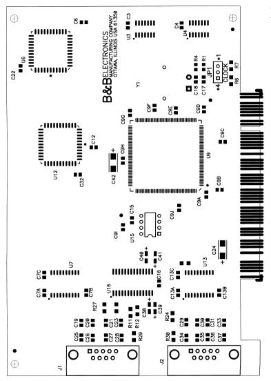
Figure 1. Silk Screen Plot of 232PClxx PCB
